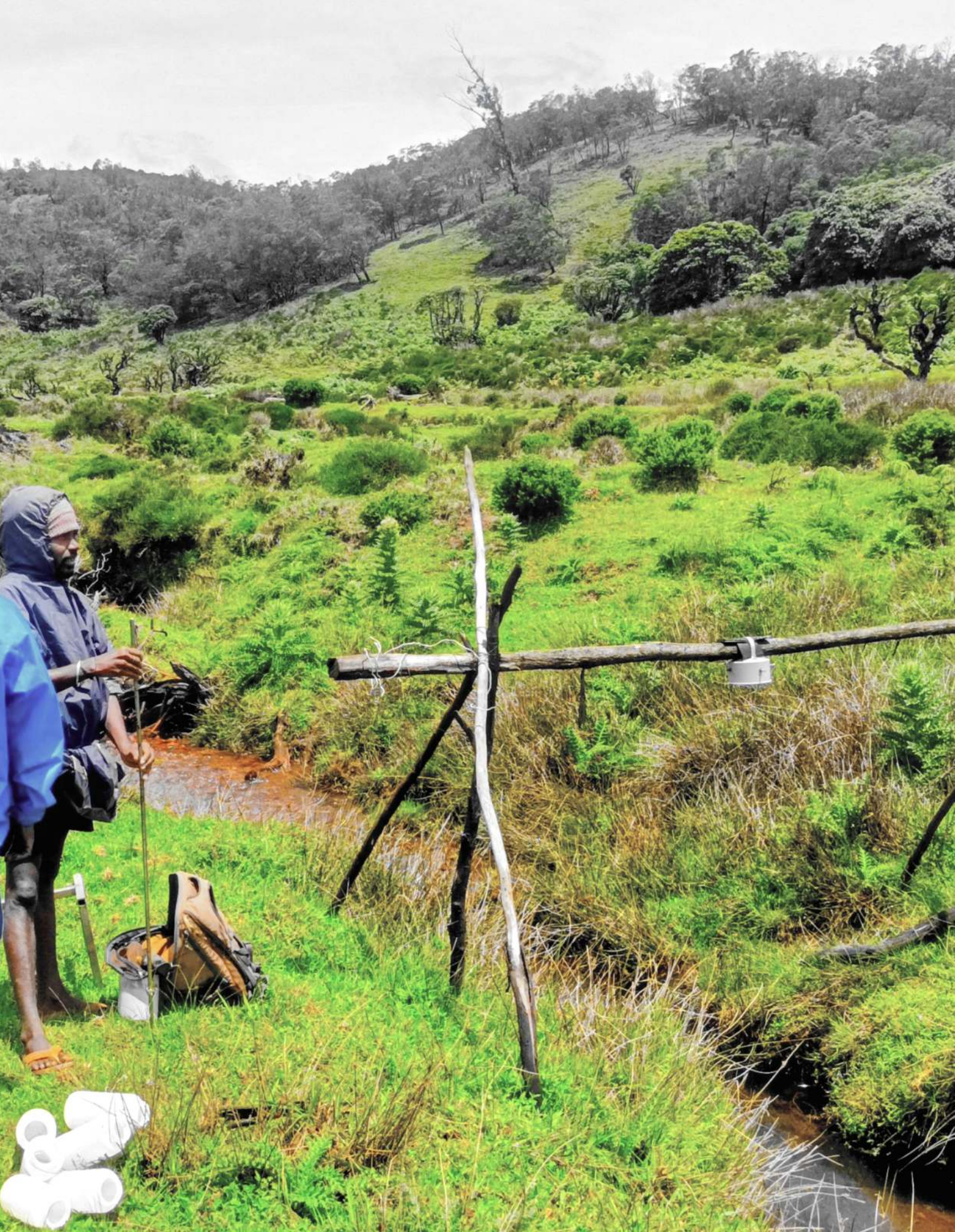
We monitored stream levels using acoustic-based water level recorders in different catchments. Regular monitoring helps in assessing seasonal changes and the impact of different vegetation cover on stream-flows.
