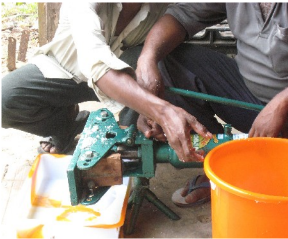
Press 4 : Spillage from the side
