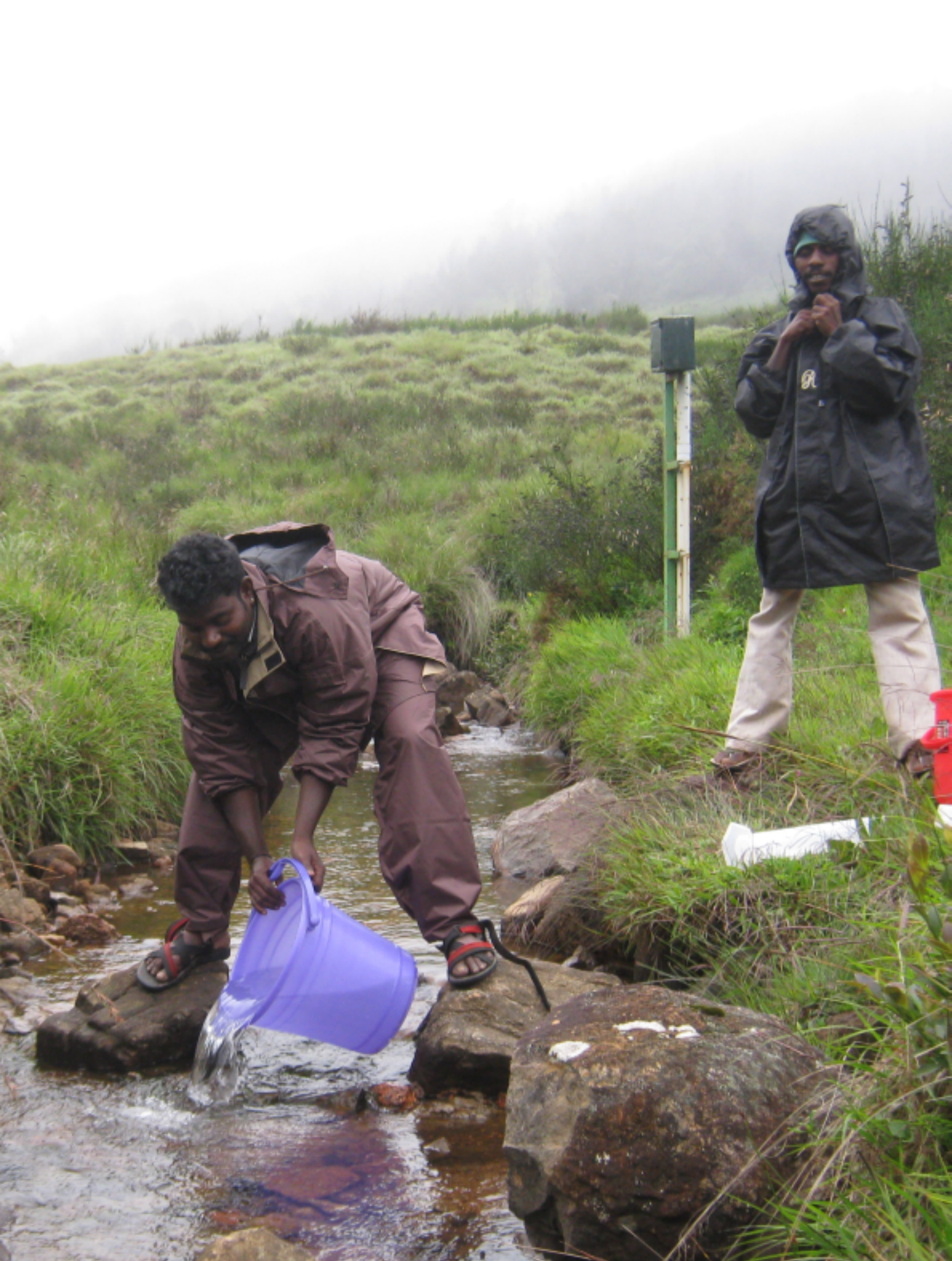
Field teams measuring stream velocity using salt dilution method.
