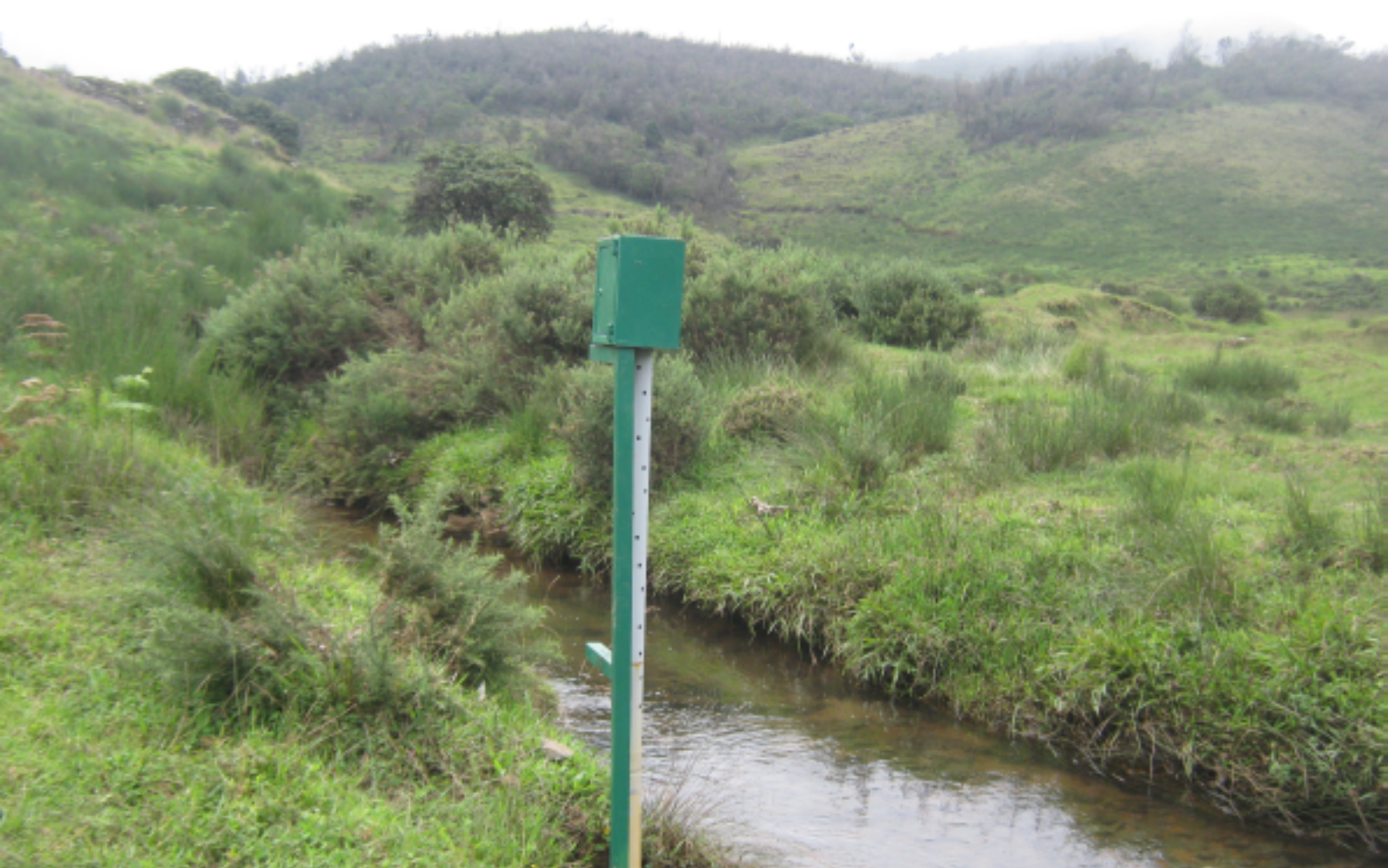
A water level recorder installed in a grassland patch dominated by invasive gorse plants.
