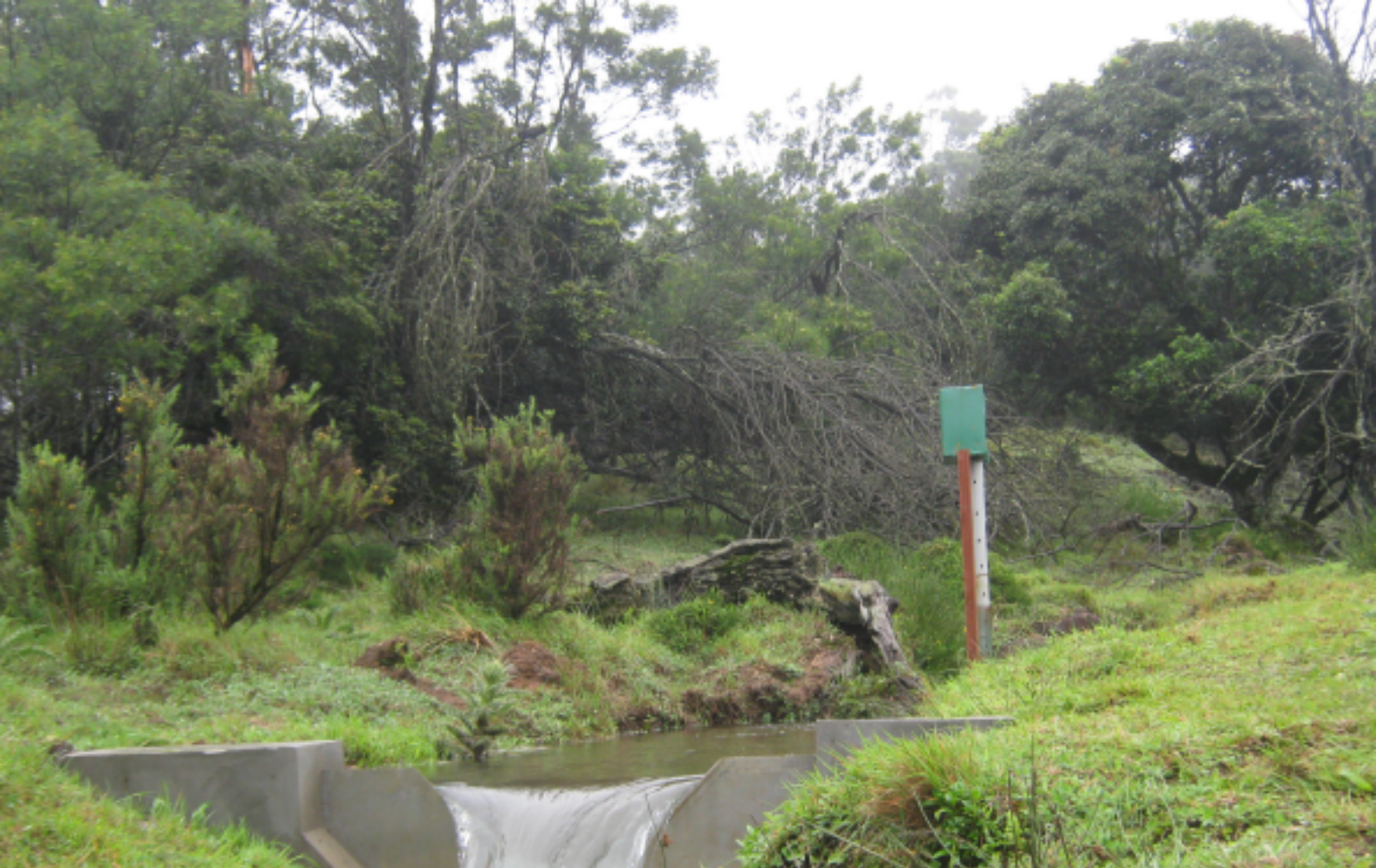
A V-notch along with water level recorder installed in a invasive wattle dominated catchment.
