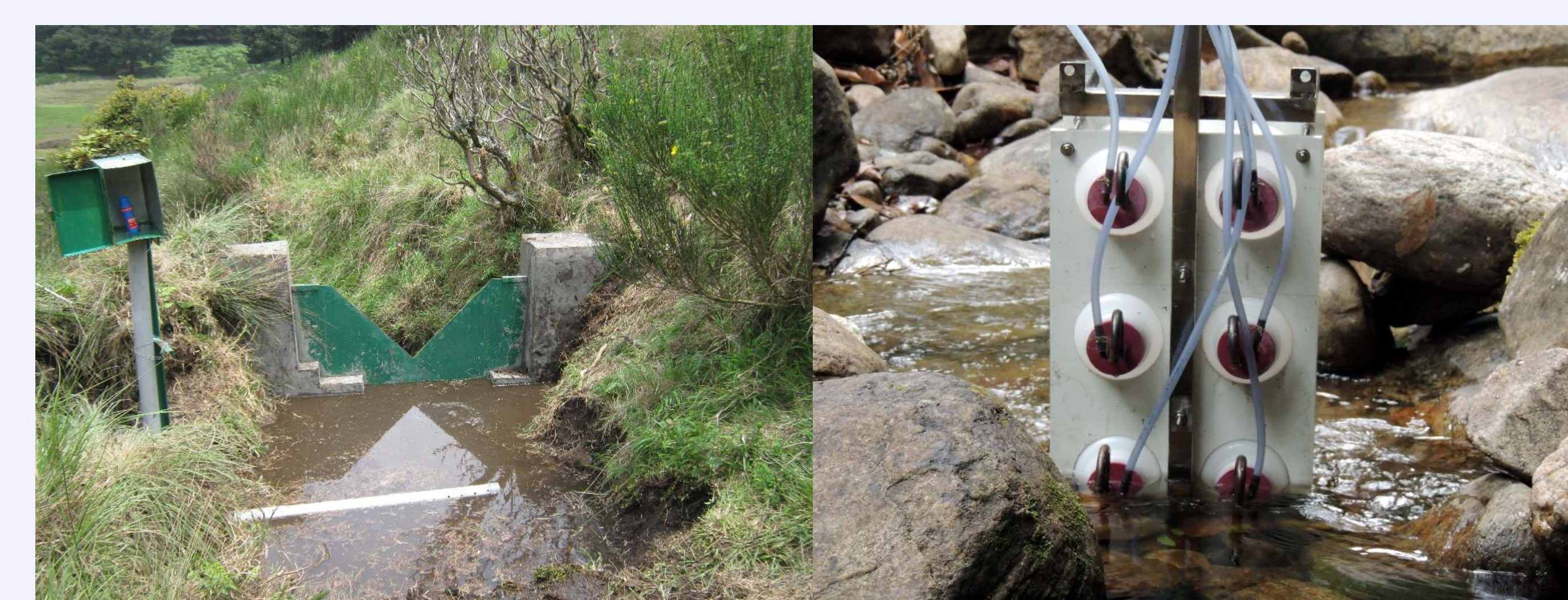
Figure 2: The weir installed at the site along with the stilling well and water level recorder (left). The stage sampler based on the USGS design used to collect samples from rising water levels of streams.
