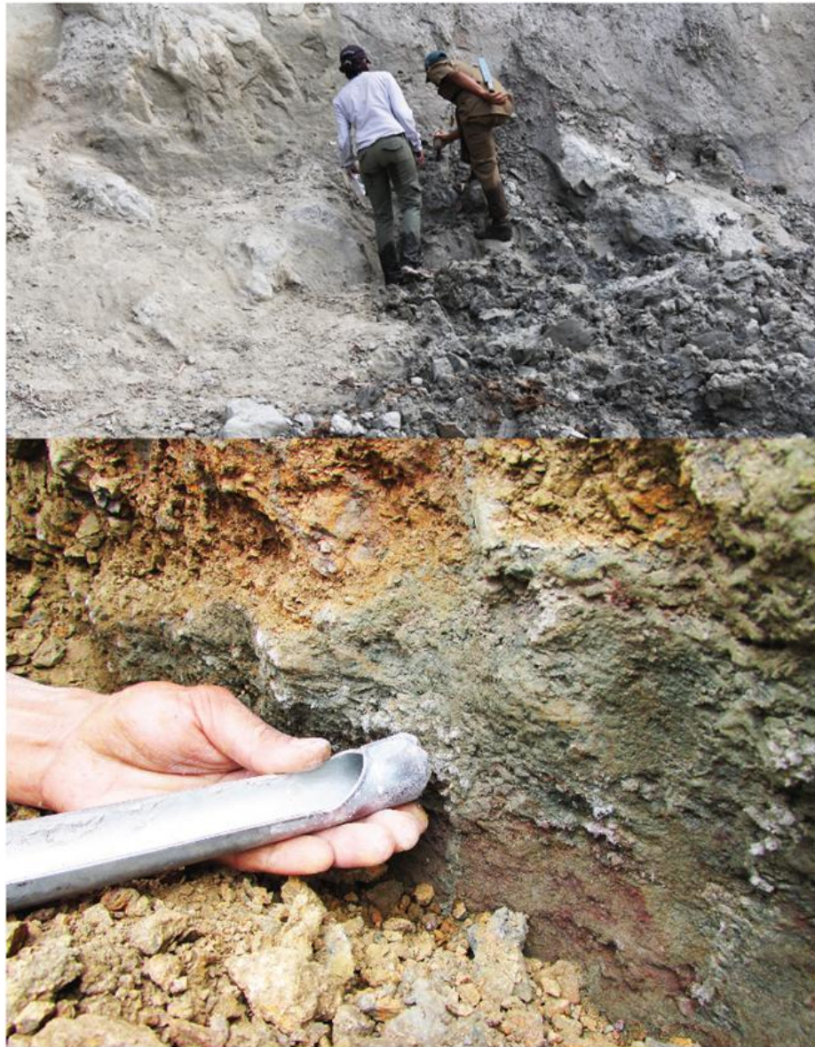
PLATE-4: Materials and methods (salt-licks) 1) Soil being collected from Dekorai saltlick for analysis of mineral composition | 2) Soil corer being used to collect soil sample from saltlick
