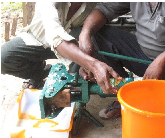
.Press 4 : Spillage from the side
