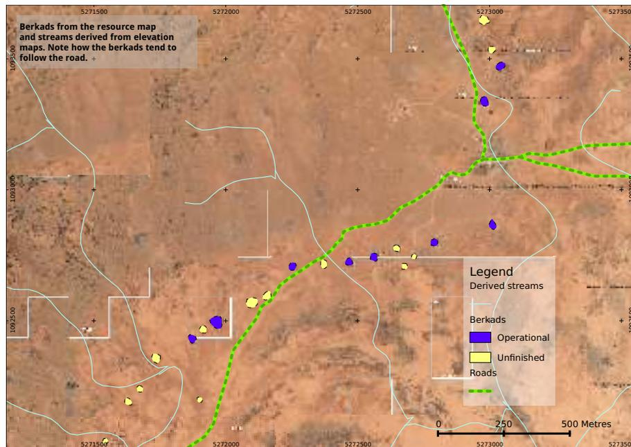
Figure 5.4: Location of berkads in relation to drainage patterns and roads. The blue coloured polygons are operational berkads while the blue lines are streams that were derived from an elevation map. The figure shows that a large number of berkads in the village are not working (yellow). Furthermore, most of the berkads located east to west are not near any drainage lines, indicating that they are not located optimally.
