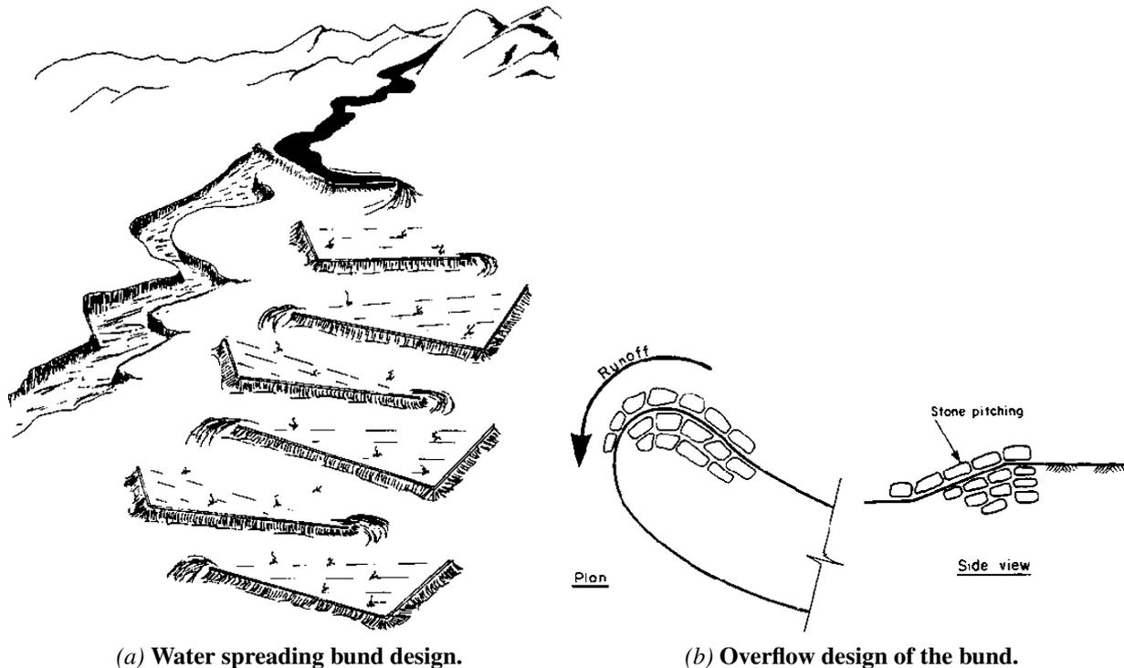
Figure 4.1: A water spreading bund, usually used in gradual slopes. The bund ensures that soil moisture is increased and soil loss arrested while it makes provision for excess water to drain. Source <http://www.fao.org/docrep/U3160E/u3160e07.htm>.
